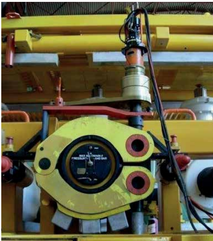
Subsea 63,000 N-m pipe clamp tool under test
